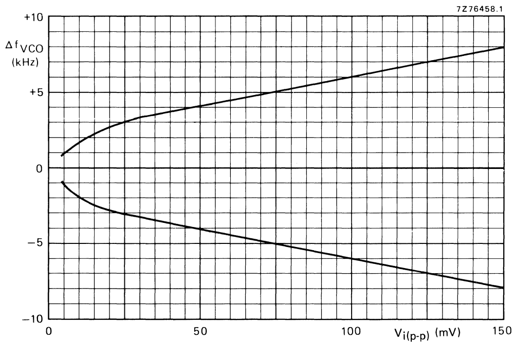
Fig. 27 Typical values of the capture range of the oscillator as a function of the pilot threshold voltage at MUX-input.
