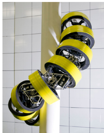
Figura 4 - Robô Hydra - Usando a pressão dos módulos para fixar ao cano - The Robotics and Mechanisms Laboratory (RoMeLa) of the College of Engineering at Virginia Tech. fonte http://www.romela.org/hydras-hyper-redundant-discrete-robotic-articulated-serpentine
